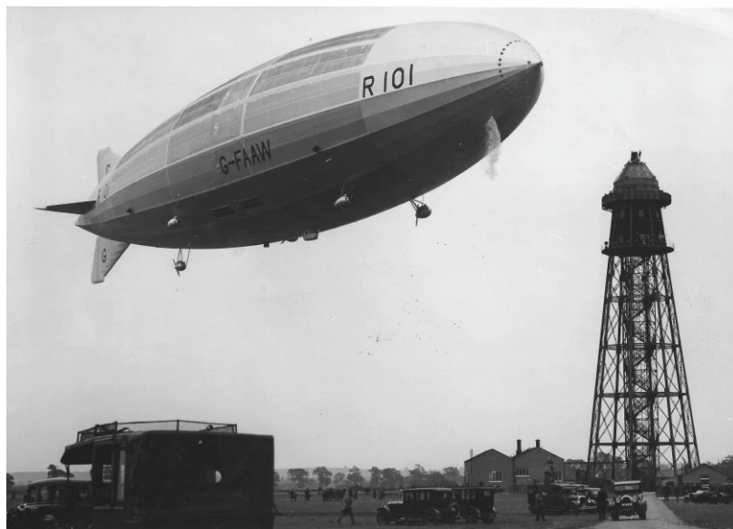
R101 discharging water ballast as it leaves the mooring mast at Cardington (Photo with permission of Alastair Lawson)
